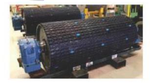
Based on this recommendation Curragh committed to a trial with three pulleys to be installed and lagged by HEME approved applicators with the Elastotec HV.
